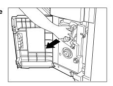
Pull out the grip of the saddle stitch holder (①) toward you and turn it (②) 90° clockwise in the direction of the arrow.
